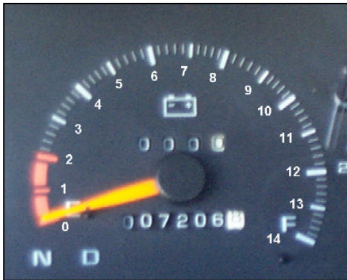
Figure 3-6. 1997 S-10 EV State-of-Charge gage
