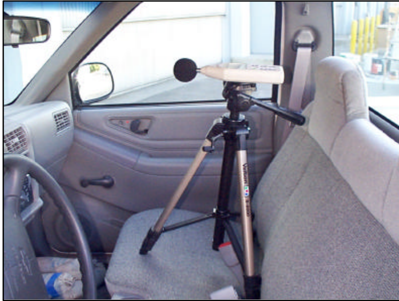
Figure 4-6. Sound level meter test setup.
