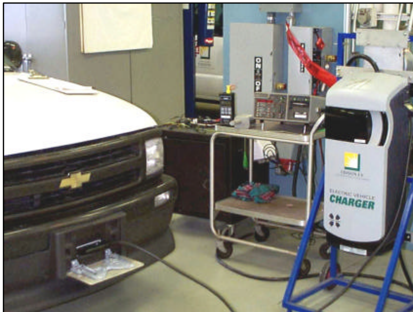
Figure 4-4. Charger testing with off-board 6.6 kW inductive charger.
