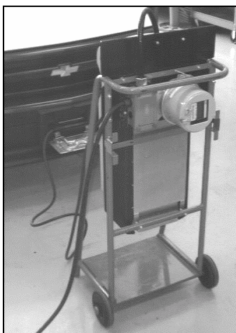
Figure 14. S-10 charger mounted on cart with ABB kWh meter.
